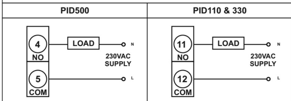
**Fig2. Output 1 - Relay / SSR to drive contactor(For single phase).**
