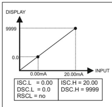
Reverse acting indication can be accomplished by setting **reverse scaling** parameter as YES. In this case **referring the above eg.** for 0.00 mA input the display will show 9999 and 20.00 mA input the display will show 0.0
