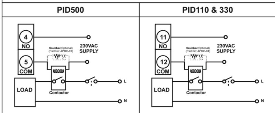
**NOTE:** Use snubber as shown above to increase life of internal relay of temperature controller.
