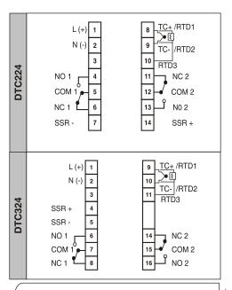
Use only the correct thermocouple wire or compensating cable from the probe to instrument terminals avoiding joints in the cable if possible.
