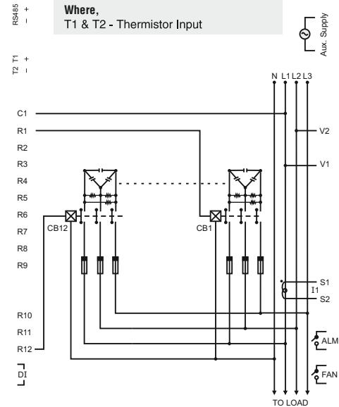
**NOTE :** • For N/W selection 2P2W voltage ( $V_{LL}$ ) applied between V1 & V2 and connect CT for I1 [ Do not use V3, N, I2 & I3 terminal ]
