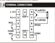
Use only the correct thermocouple wire or compensating cable from the probe to instrument terminals avoiding joints in the cable if possible.
