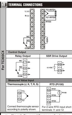
Use only the correct thermocouple wire or compensating cable from the probe to instrument terminals avoiding joints in the cable if possible. Failure to use the correct wire type will lead to
