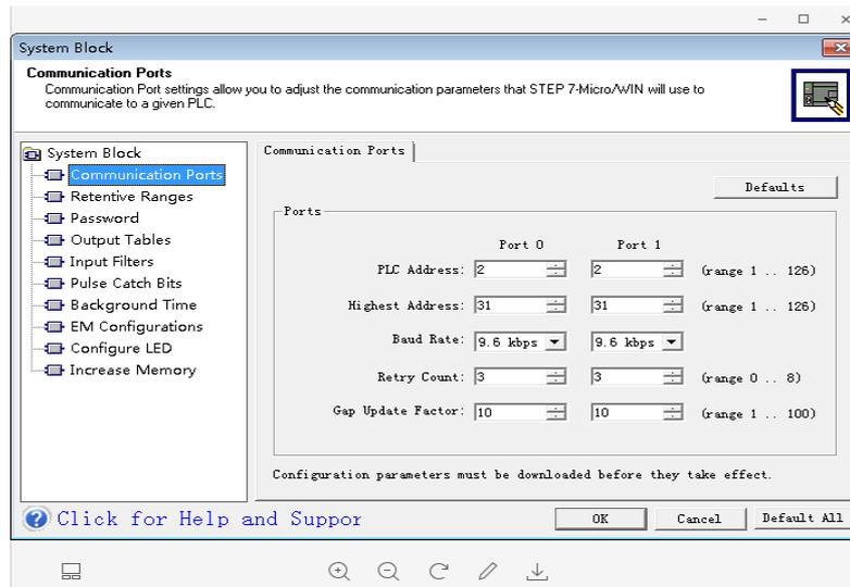
5. Connect the HMI to PLC through 485 communication cable and power them together, then download the corresponding project to HMI. When click the components on the screen, the corresponding PLC output points will be lighten.
