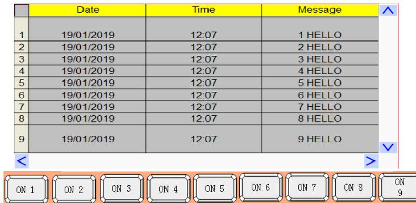
Add a dynamic alarm bar at the scene and trigger the corresponding event, the triggered time will scrolling display on the scene.
