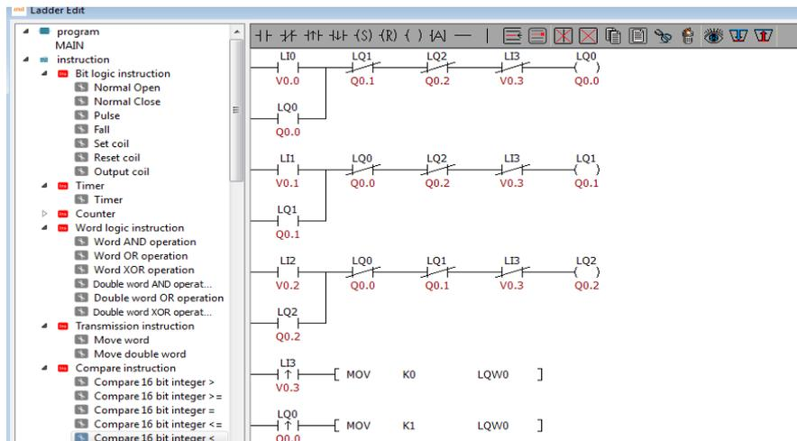
After editing the ladder diagram, the relevant controls can be placed in the screen, and the relevant logic is already operation.
