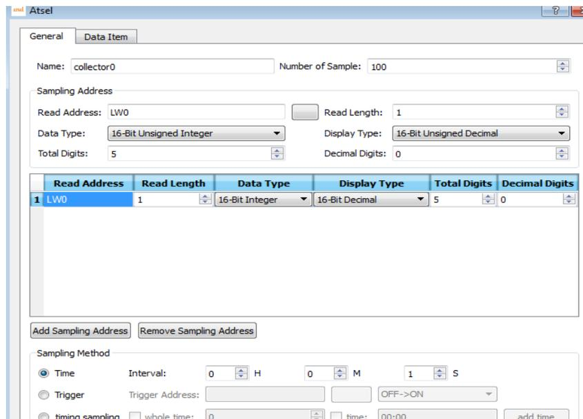
3. When the historical data collecting address is set up, you need to add the corresponding historical data display components in the software advanced options,
