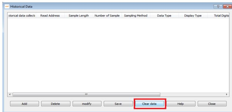
2. It controls the suspension sampling or clear historical data by address variables. Set the corresponding control address the corresponding state of the address variable is triggered the relevant function.
