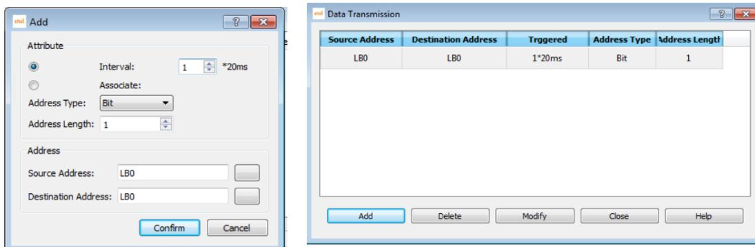
3. After adding, click close button exit, after downloading the configuration you can do data exchange according to the set transmission type.
