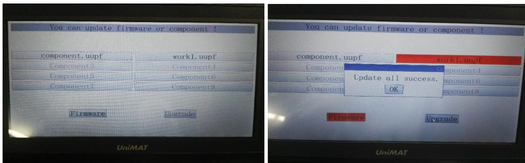
7. Pull out the U disk and restart the touch screen to complete the U disk update.
