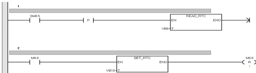
B. Add 8 numerical inputs in ATSEL as PLC time display, the data type is 16 bit BCD code, address is VB0~VB7.
