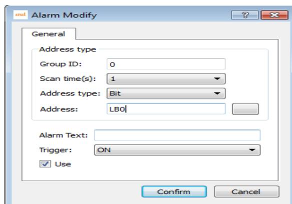
3. Add an alarm control, and change the corresponding display parameters.
