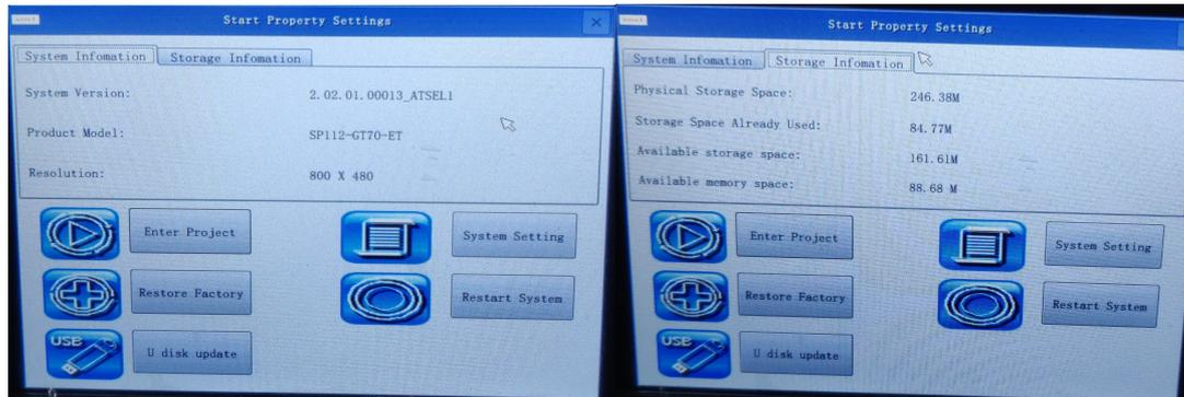
System settings, in the system settings, you can view the current system information, including the current application software version number, version type, and the IP address of the machine (if no Ethernet shows no support); can adjust the back-light brightness through a scroll bar; in calibration, the touch screen can be calibrated; IP The address can set the IP of the Ethernet HMI.
