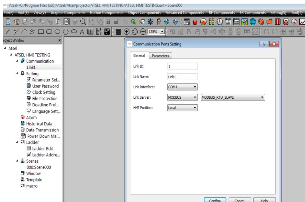
2. PPI communication parameters setting as showing in below chart.
