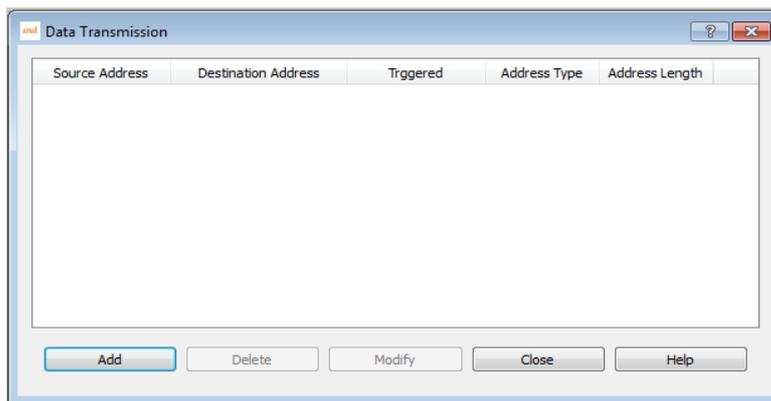
1. Click "Add", you can add data transmission. At present, maximum number entries is 100. Triggered type is interval trigger and minimum time unit is 200ms, the data types which can be transferred is bit, word, double word, and the maximum transmission data size by each trigger is 100(bit, word, double word)
